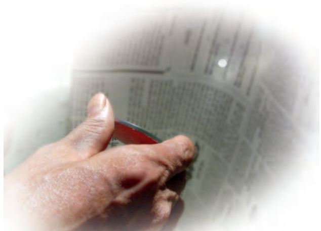
Fig. 11.14 A concave mirror forms a real image of the sun
